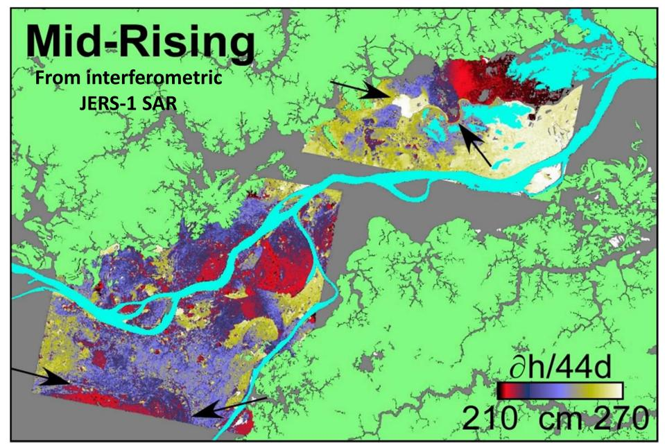
In densely forested environments, L-band (and other wavelength) SARs can be used to measure water surface elevation using double bounce.
