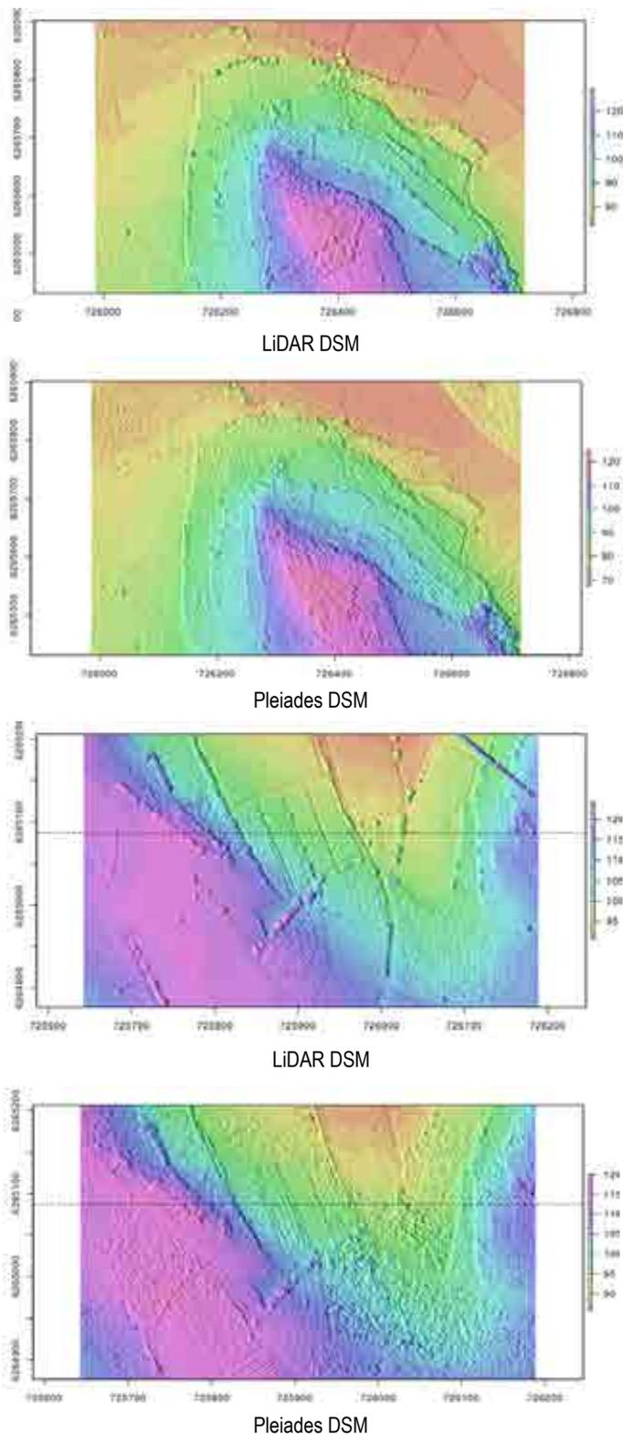
Fig 1. (a) 2 zooms on the LiDAR and Pleiades 1 m DSMs on the Peyne river basin
