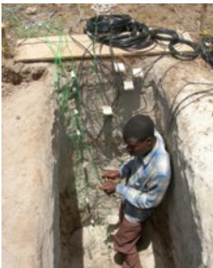
Measurement of the soil humidity and temperature profile in Benin © S.Galle
