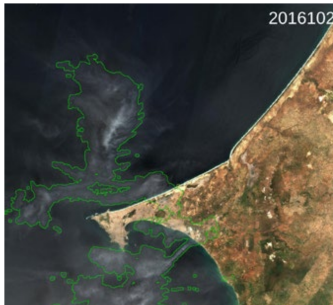
Example of a level 2A product for Dakar, Senegal. The clouds that were detected are marked in green.
