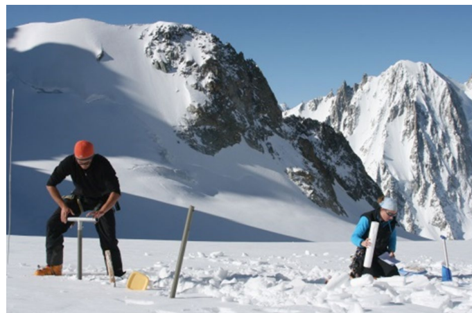
Measurement of the Glacier du Tour Noir: winter review based on ice cores and snow density measurements, France, April 2013 © Patrick Ginot.
