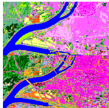
Comparison between land cover maps generated using Landsat 8 data (top) and Sentinel 2 (bottom) on the Rhone, the Durance and the city of Avignon
