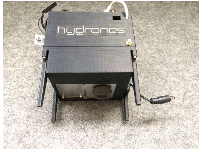
Figure 2 : HyDrones #MK2 prototype dedicated to bathymetry
