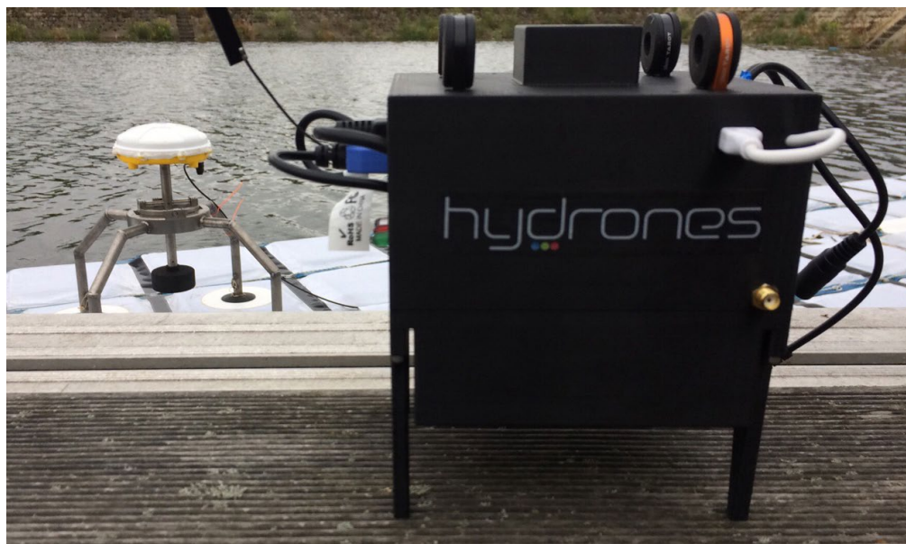
Figure 1 : Prototype of HyDrones #MK1.1 light altimeter. In the background: «CalNa-Geo» GPS carpet
