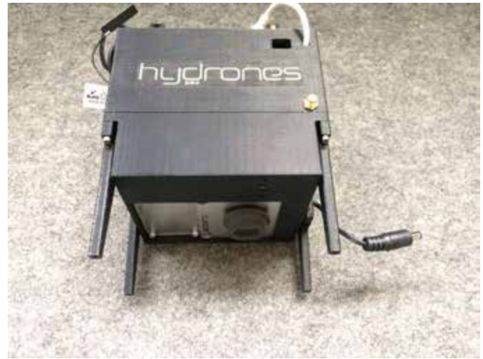
Figure 2 : HyDrones #MK2 prototype dedicated to bathymetry
