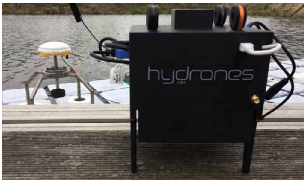
Figure 1 : Prototype of HyDrones #MK1.1 light altimeter. In the background: «CalNa-Geo» GPS carpet
