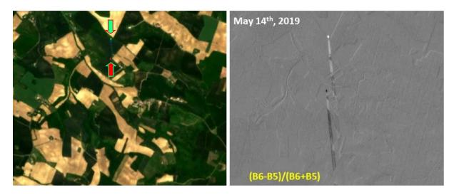
Example of information derived from stereoscopic and time lag features: left a RGB composite of B7, B4, B3) where the green and red small dots are the same airplane within a few tenth of seconds. On the right, a combination of bands B6 and B5 enhance the change in the location of the plane and its contrails (an additional effect is the rotation of the Earth).
