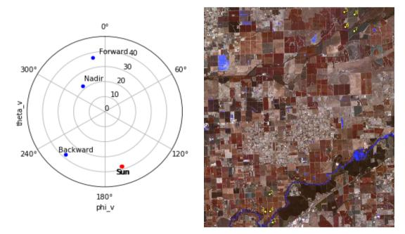
Example of multi-angular acquisitions acquired from the same orbit in a few minutes. On the left geometric configuration, on the right RGB colored composition using the same spectral band (B6 = 620 nm) acquired in three directions. Forward sight in blue, "nadir" green, backward sight in red. Water appears blue due to specular reflection. The vines whose rows are oriented East-West appear in burgundy color, those oriented North-South appear in gray. (more <a href="here">here</a>)
