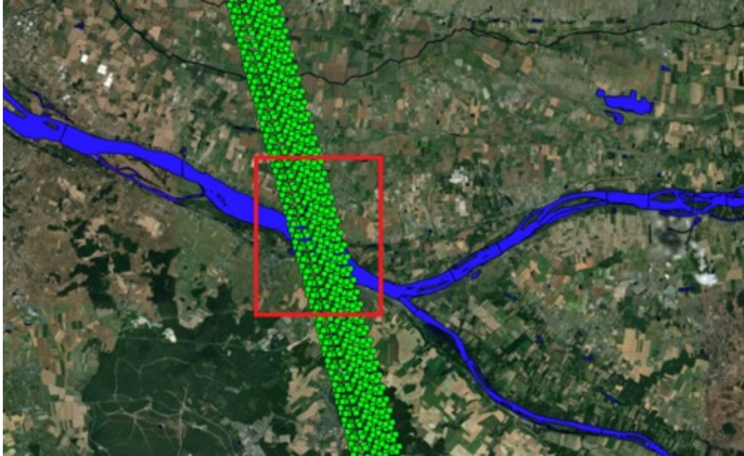
Figure 4: Virtual station concept. Example over the Loire river with Sentinel-3A. 20 Hz measurements are represented in green points (several cycles for a same pass number). An example of virtual station geographical area is shown as a red rectangle
