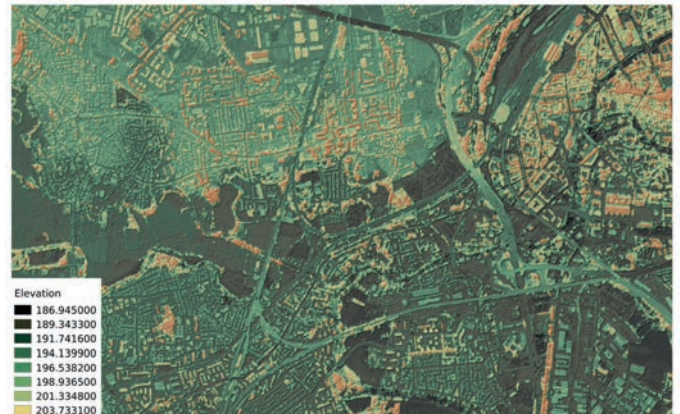
Figure 2. Example of a digital urban surface model generated for the city of Strasbourg (Grand-Est) in the framework of THEIA Urban SEC activities (© A. Puissant & A. Stumpf, LIVE/THEIA)
