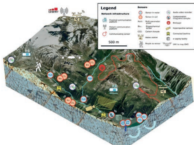
Schematic illustration of what a TERRA FORMA observatory could be, a site combining fixed and mobile communicating sensors and communication platforms © Virginie Girard, Laurent Longuevergne, Arnaud Elger
