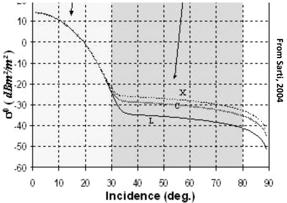
semi-empirical function of backscatter coefficient  $\sigma^0$  as a function of incidence (for a mean sea), for 3 different radar bands
