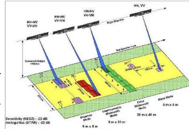
Figure 129: Overview of the Sentinel-1 C-SAR instrument observation scheme and operational support (image credit: ESA)
