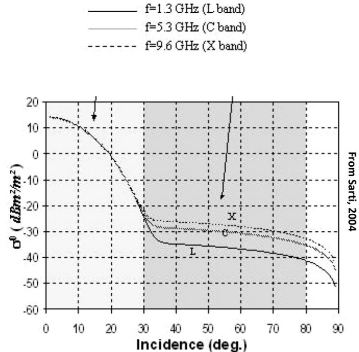
semi-empirical function of backscatter coefficient  $\sigma^0$
